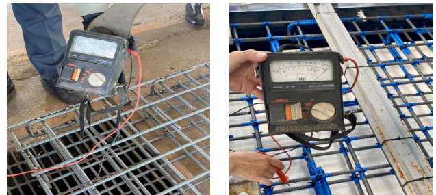
Fig. 5. Normal rebar (Right) and Insulated rebar (Left).
